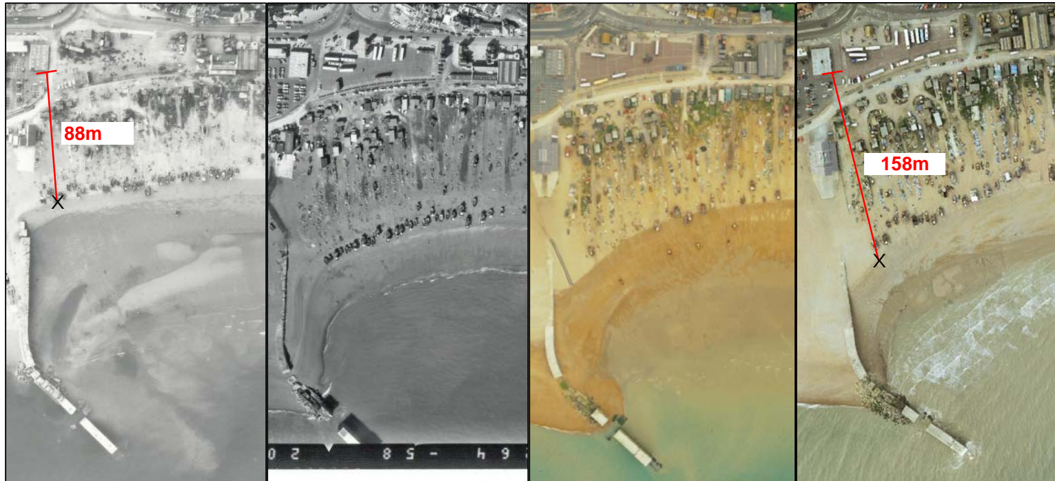
Figure 5.3: Beach Width Changes from 1980-2008. The distance between the front of a building beside the coach park and the beach crest has been measured for both the 1980 and 2008 aerials in order to see how far the beach has advanced over that time period.
