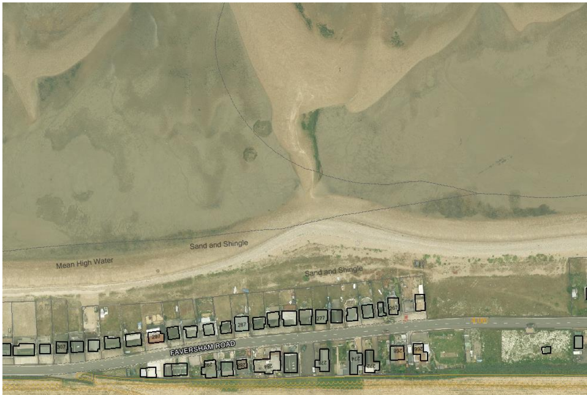
FIGURE 8-2 FAVERSHAM ROAD PROPERTIES AND THE SHINGLE BAR WHICH IS TRANSGRESSING ONSHORE © CROWN COPYRIGHT AND DATABASE RIGHTS 2016 ORDNANCE SURVEY 100019614. AERIAL PHOTOGRAPHY ©CHANNEL COASTAL OBSERVATORY.
