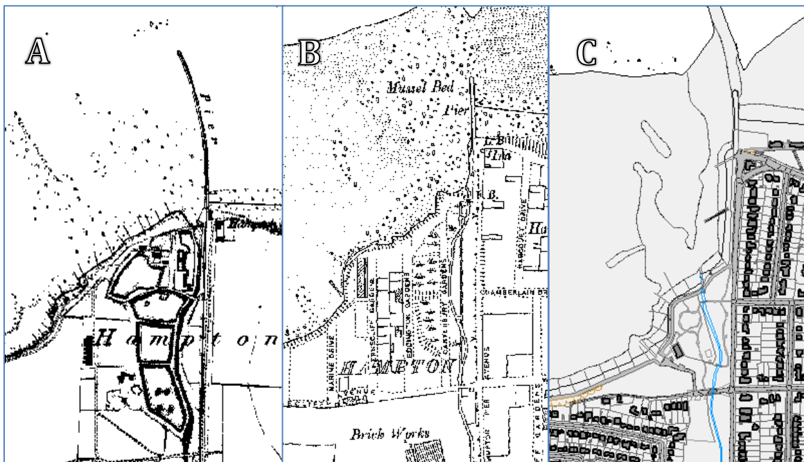
FIGURE 1-21 EROSION CAUSED BY THE CONSTRUCTION OF HAMPTON PIER: A – HAMPTON IN 1872, B – HAMPTON IN 1910 AND C – HAMPTON TODAY
