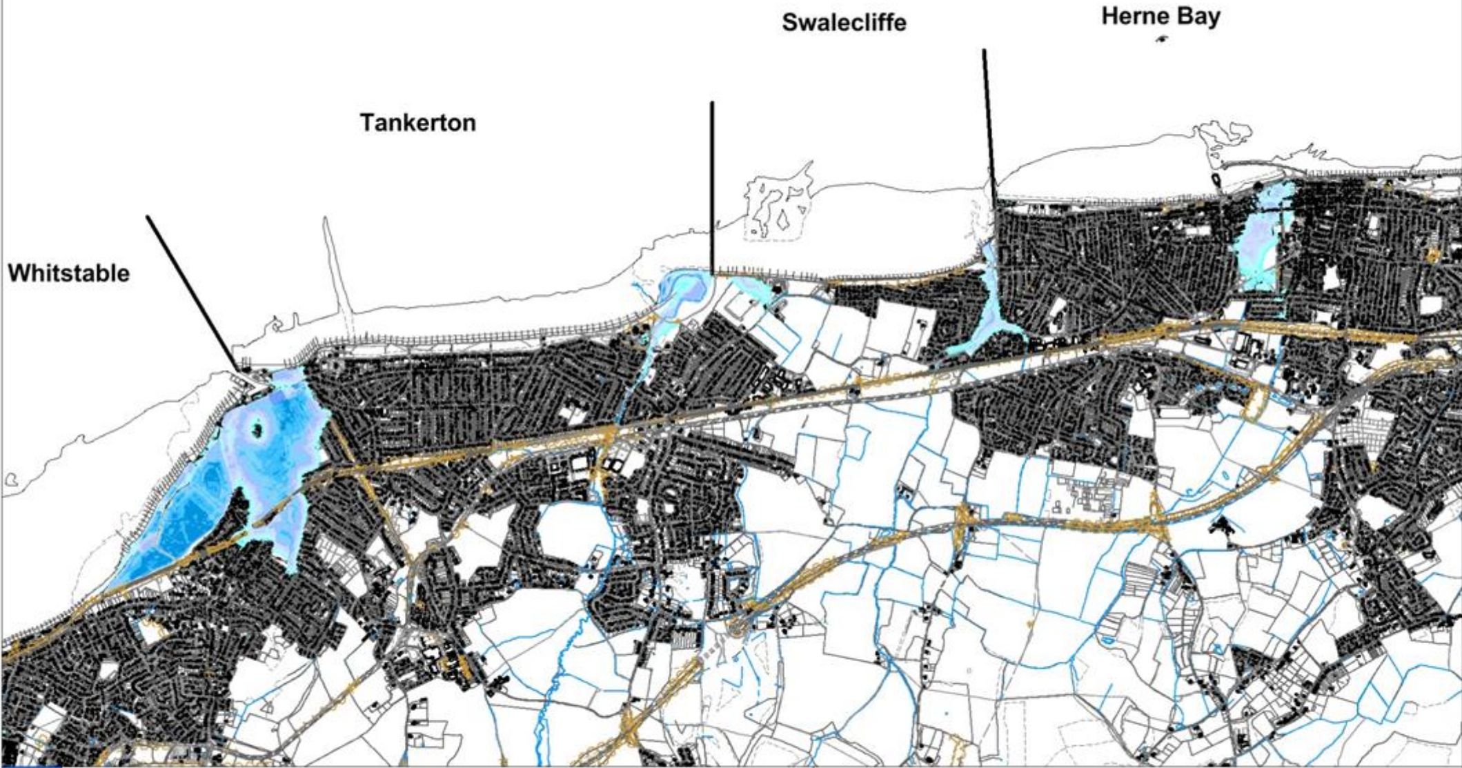
FIGURE 2-2 WHITSTABLE TO HERNE BAY FLOOD DEPTH FOR 1 IN 200 YEAR STILL WATER LEVEL (PLANAR FLOOD MAP)
