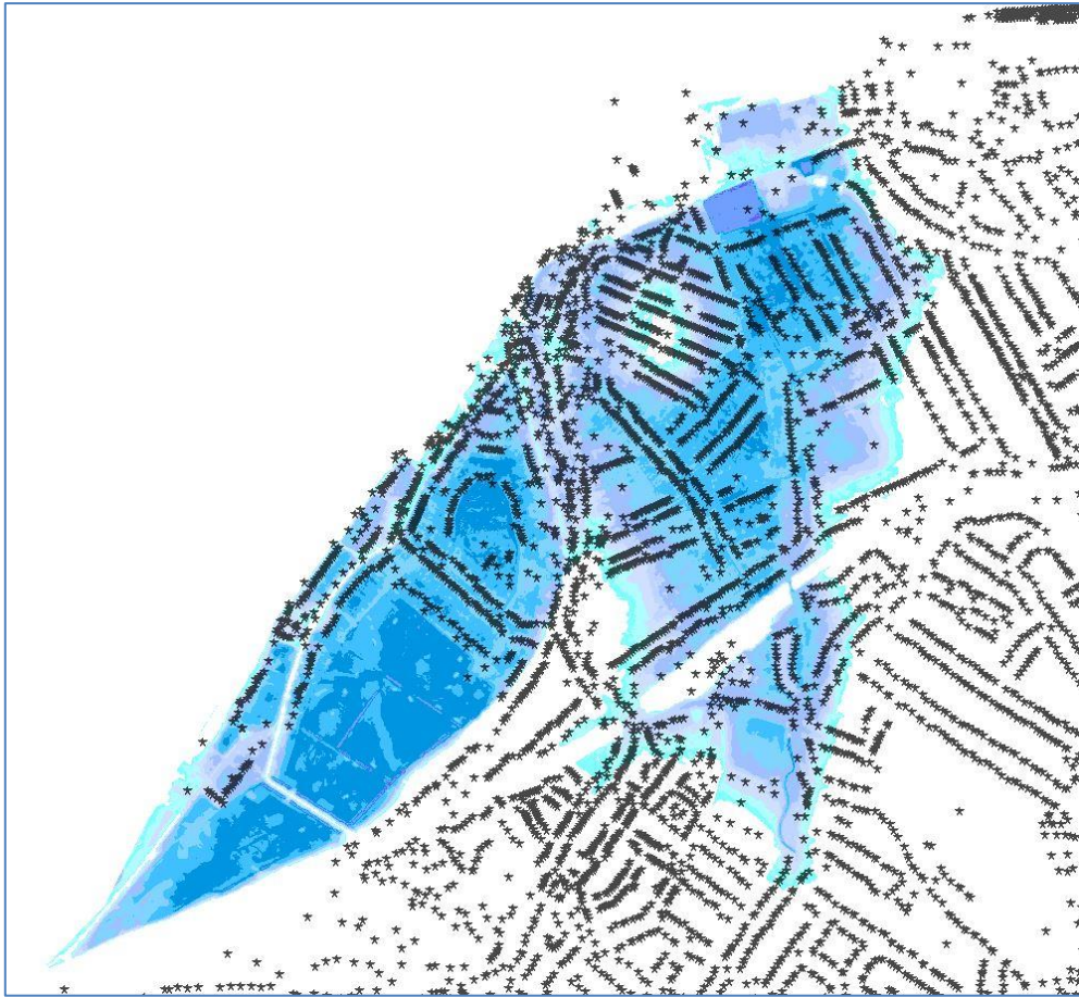
FIGURE 62-20 EXAMPLE OF PROPERTIES (STARS) IN WHITSTABLE WITHIN THE 1:200 YEAR EXTREME WATER LEVEL PLANAR FLOODPLAIN
