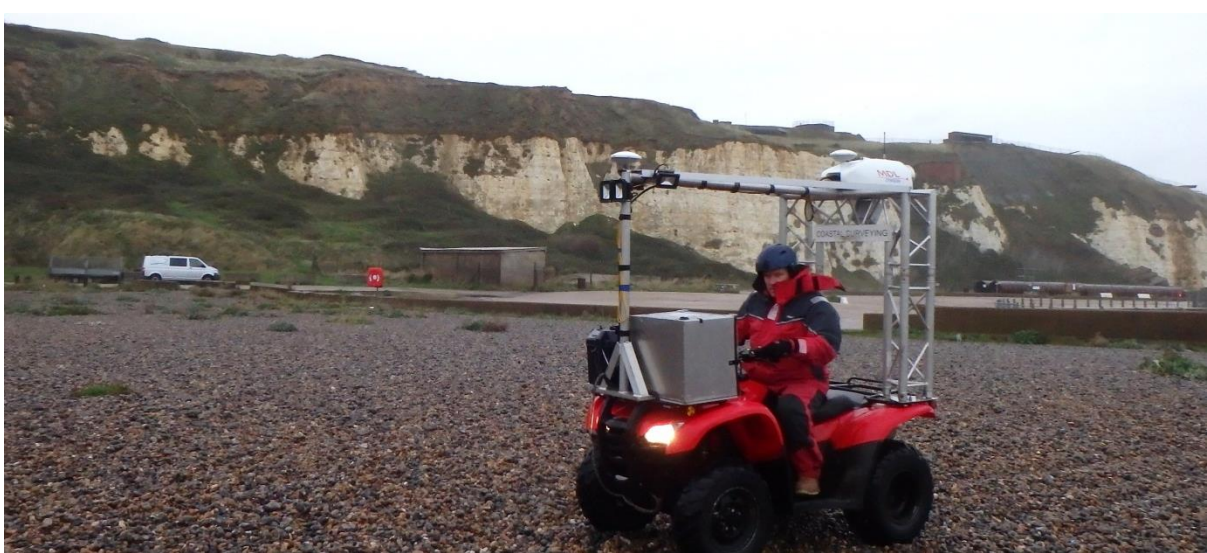
FIGURE 9-1 MOBILE LASER SCAN MOUNTED ON AN ATV – HASTINGS (2012)
